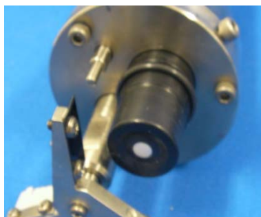
Galvanic type sensor (COMPACT-DOW)
